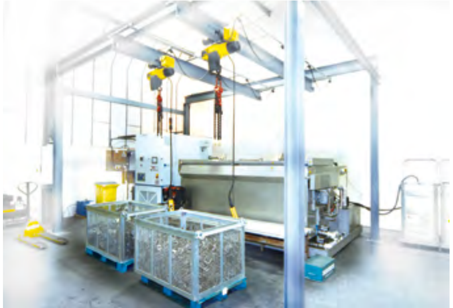
fig. 2 GIGANT TOP-LOADER with double gantry crane
